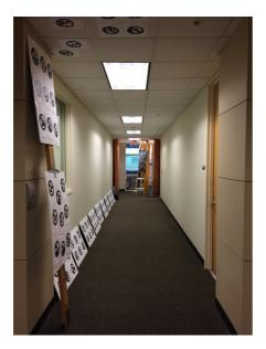
Figure 3. Indoor localization testing, using the mounted fiducials for the Intersense IS-1500 tracking system.
